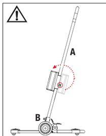
A. Push the rising ladder/tube down into the mounting fixtures on the chassis, so that the height-adjustment buttons are facing towards the caregiver.
