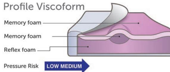
The profile version of the Viscoform cushion provides aommel, which can support those with weak trunk or lower limb muscles who are prone to sliding down and forward in their chair or for those with lower limb spasticity to help maintain hips in the abducted position to create a good seating position.
