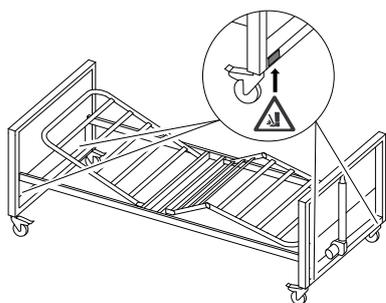
1. Place the four foot squeezing warning labels (delivered separately) on the lower sides of the bed ends near the castors.
