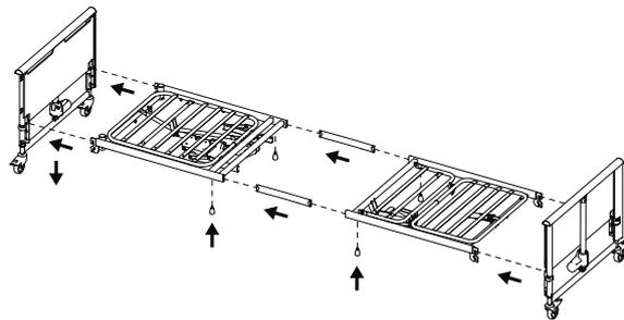
1. Place the two inserts in the upper half of the mattress support. The inserts must be mounted in such a way that one extends further out of the side tube than the other.
