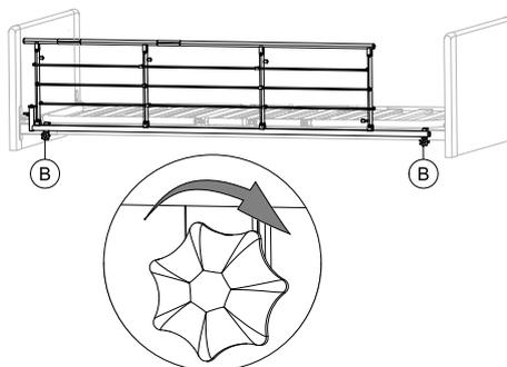
Tighten the finger screws **B** to attach the side rail on the top frame. Make sure it is steady and fastened.
