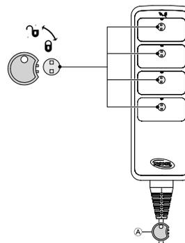
1. Insert key ① in the keyhole located just above the desired function.
