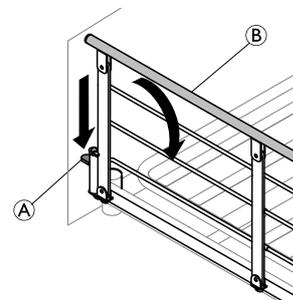
1. **Up:** Lift and pull the top bar ② of the side rail towards the end with the locking mechanism (release button) ①. Ensure, it is locked in place.
