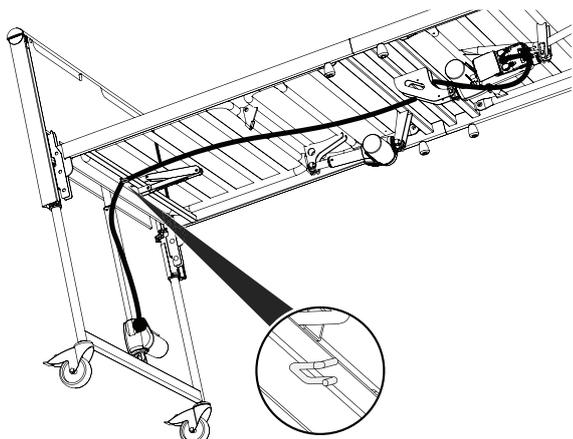
10. Guide the mains cable through the frame hooks on the side of the bed to the power outlet and connect it.
