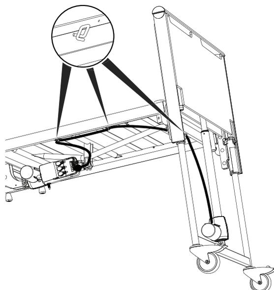
8. Disconnect the foot Hi/Lo motor cable from the control box, guide it through the opening of the support for the backrest motor and reconnect it.
