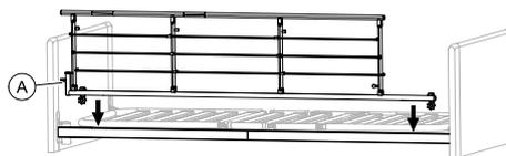
Place the side rail over the top frame with the release system **A** at the head end of the bed.
