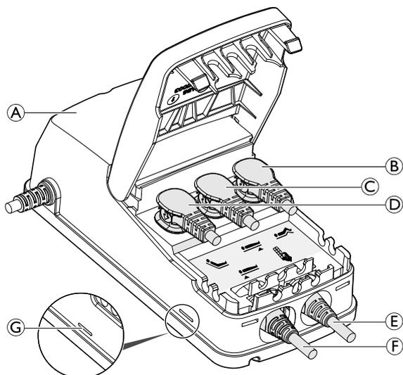
The control box **A** is provided with a label with symbols showing where to connect the motor plugs:
