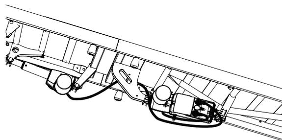
7. Guide the head Hi/Lo motor cable through the frame hooks on the side of the bed and the end of the coiled part on the bed end hook.
