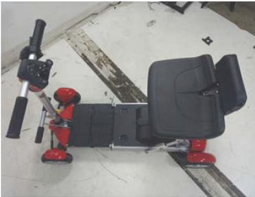
10. Pull the yellow knob back to the rear support bar. (Folding up the scooter part 1)
