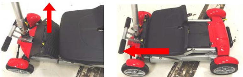
7. Use slide lever down for suitable location. (Folding up the scooter part 4)
