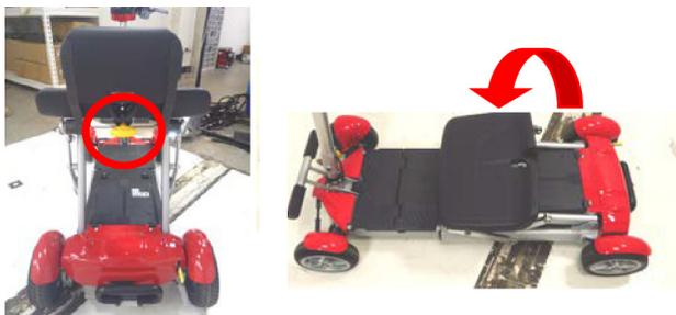
6. Push up the pedal, position the pedal plate forward. (Folding up the scooter part 2)
