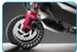
Shock-absorbing airless NPT tires
