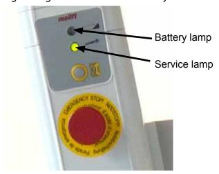
The electronics logs how much the lifter is being used, and the load it is used with. After a given time of usage there will be given a signal that the lifter needs service to the service LED. The LED will first give a yellow light, then red. Take contact with your local service representative and order service. If there is a sound together with the light, it means the lifter needs service immediately.
