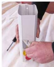
• Pull the three parts of the battery support carefully apart.
