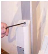
Disconnect the cables on the backside of the battery support.
