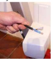
Open special screw B<sup>®</sup> at the lower actuator bracket **B**<sup>®</sup> using the special wrench.
