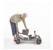
Fold the steering column down by first loosening the tiller adjustment knob and then slowly pushing the steering column down towards the base plate. Once the steering column rests on the bottom plate, tighten the tiller adjustment knob to hold it in place.
