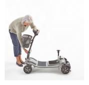
Lift the steering column up by first loosening the tiller adjustment knob and then slowly lifting the steering column up, away from the base plate. Once the steering column is upright, tighten the tiller adjustment knob to hold it in place.
