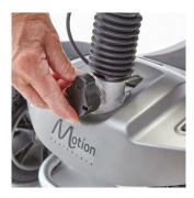
Lock the steering column in place using the steering lock by pressing the lock and turning it 90 degrees clockwise.
