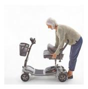
Slide the seat onto the seat post. Always check and make sure the seat is securely fastened before sitting on it.
