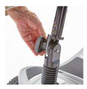
To adjust the steering column, hold the steering column with one hand and, with the other hand, turn the steering column adjustment knob anti-clockwise until the teeth unlock and the steering column moves up and down freely.
