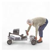
Lift the rear section removal handle with one hand and pull the rear section down with the handle to separate the front and rear sections. Lift the front section up and away.
