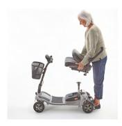
Raise the seat rotation lever and lift the seat to remove it.
