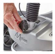
Unlock the steering by pressing the lock and turning it 90 degrees anti-clockwise.
