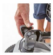
When the steering column is in the desired position, turn the steering column adjustment knob clockwise until it is as tight as possible.
