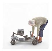
Use one hand to pull down the rear section with the handle and lift the front section using either the seat post or rear section removal handle. Drop the front section into the rear section and push down until you hear a click. Always check that the sections are connected correctly before moving on to the next stage.
