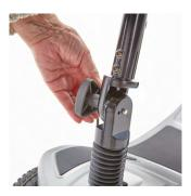
To adjust the steering column, hold the steering column with one hand and, with the other hand, turn the steering column adjustment knob anti-clockwise until the teeth unlock and the steering column moves up and down freely.
