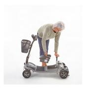
Use the handle on the battery to lift up to remove the battery pack. Be aware that the battery is secured in place with Velcro, so if you have trouble removing it, press on the seat post to make it easier.
