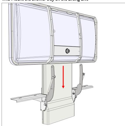
Slide the shower tray in between the lifting unit and the support arms on the lifting unit. It is an advantage to be two persons when doing this.
