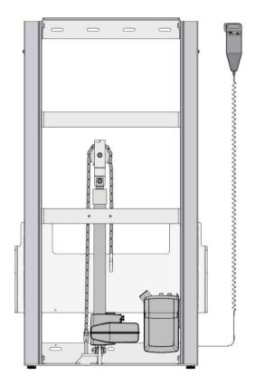
All the plugs are watertight, and therefore they can be a little tricky to connect / disconnect. Make sure that the plugs are positioned correctly before they are pushed into the sockets at the control box. The plugs must be pushed into the sockets until the "O-ring" is no longer visible.
