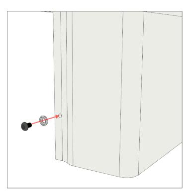
When all the wires have been attached and screws fastened, the cover must be fixed in place. Use the attached M5x8 screws and screw button cover. This step can wait until the end to make it easier to access the control box and wires if needed.
