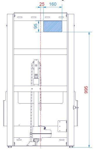
The following drawing illustrates the space that can be allocated for an electrical outlet without interfering with the movement of the unit. The blue-hatched area are is the safe area for placing an electrical outlet and cover. Placing the outlet and/or cover outside of this area may result in product damage and malfunction.
