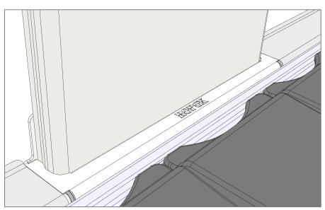
Double check that it sits flush and fiirmly on the lifting unit
