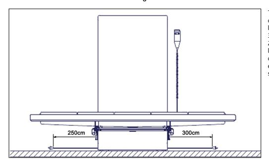
The main power cable has a total length of approx. 320cm of which 250cm is outside the lifting unit. The cable can be pulled out in either left or right side.
