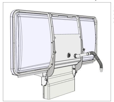
Screw the plastic nut on the scuttle and tighteen it firmly. Connect the flexible hose to the drain tube and connect it to the drain in the wall or on the floor.
