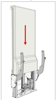
The cover can either be clicked in place from the front or slide down from above. Make sure that the cover reaches the floor and is in contact with the wall at the top. This step can also wait until the end of the installation process if ease of access to the electrical components is required.
