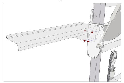
Use 4 pcs. M6x6 screws to mount the shelves on both sides of the lifting unit.
