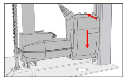
To gain access to all the bottom holes, the control box will need to be temporarily removed. This is done by unlocking it from the holder at the top, pressing it back and sliding the control box down.
