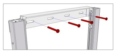
Maximum pull force for each of the four screws in top of the unit: 45 kg
