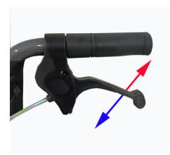
Push the brake handle down (as shown by the blue arrow) to lock the brake onto the wheel. If you wish to use the brake to slow the wheelchair when moving down a slope or incline, then pull the handle up. (As shown by the red arrow) If the brake is locked onto the rear wheel, then pull the handle up (as shown by the red arrow) to release the brake from the locked position. Both brakes **must** be locked when the user is getting into or out of the wheelchair.
