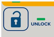
**Locking Function** - The THEIA/2 control unit will automatically lockout all functionality 5 minutes after a function change. To unlock the control unit the 'unlock' button is pressed for 3 seconds. When locked the LED indicator illuminates green.
