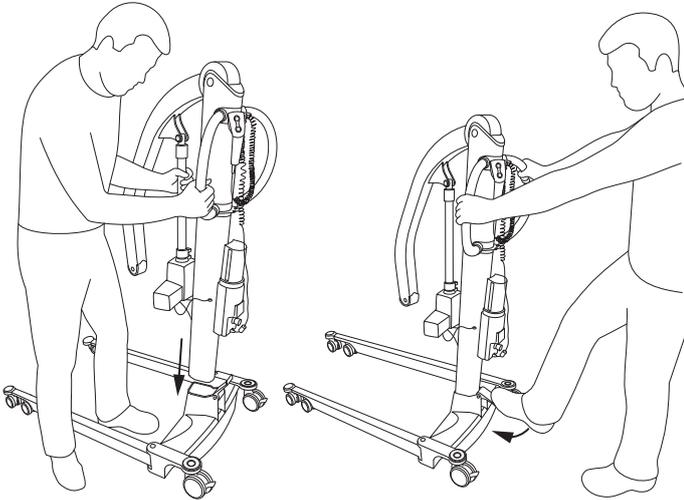
Place lifting column in chassis. Make sure that the red arrow on the lower part of the column corresponds with the edge of chassis. Make sure screw on column is inside the hole on chassis. This will prevent the column from unintentionally being lifted out of chassis when lock handle is pushed down.
