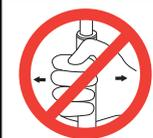
**Do not push or pull the user, lifting arm or actuator. This may cause stability problems and lifter may tip over.**
