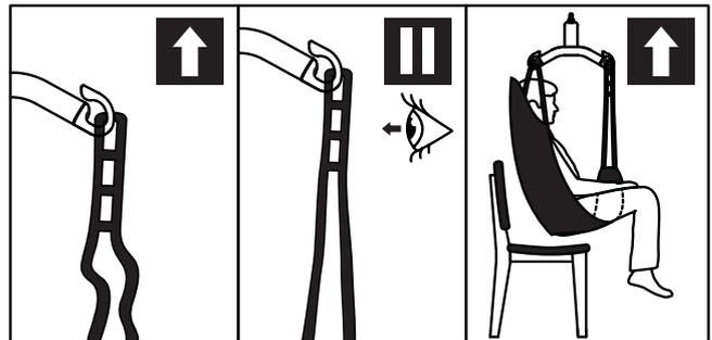
1. Check that the sling is correctly fitted around the user and that the strap loops are correctly fitted to the sling bar hooks.
