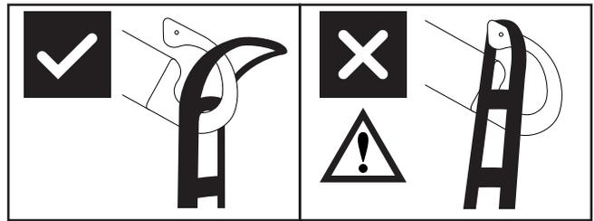
The sling bar's hook design prevents sling to be inadvertently detached when mounted correct.
