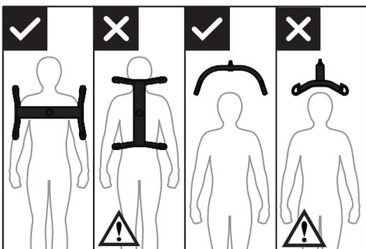
The sling bar must always be positioned across the user, to prevent the user from unintentionally sliding out of the sling.
