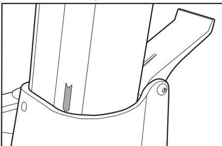
Fix the column by pushing the lock handle on the back all the way down.
