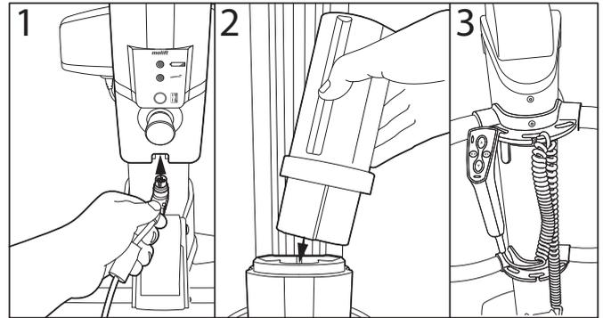
1. Connect hand control to bottom of battery holder.
