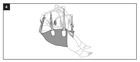
Next, attach the hip straps to the centre hooks using the nearest possible loop. If it helps, you may lift/raise the client slightly off the surface until the leg and shoulder straps are tensioned, before attaching the hip straps.
