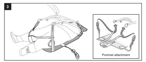
Move the lift into position above the client, keeping the cradle hooks away from the client's face. Attach the shoulder and leg straps to the respective front and rear hooks on the cradle, ensuring to feed each leg strap through the corresponding pommel loop (see diagram above). Adjust the head support to suit client comfort.
